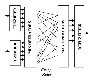
Fig. 3 Block Diagram of Fuzzy System
